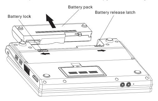
Figure 4-1 Removing the battery pack
